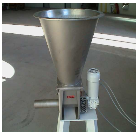
EMCEtechnix GLD 87 with hopper and metering helix (intromitter hidden)
